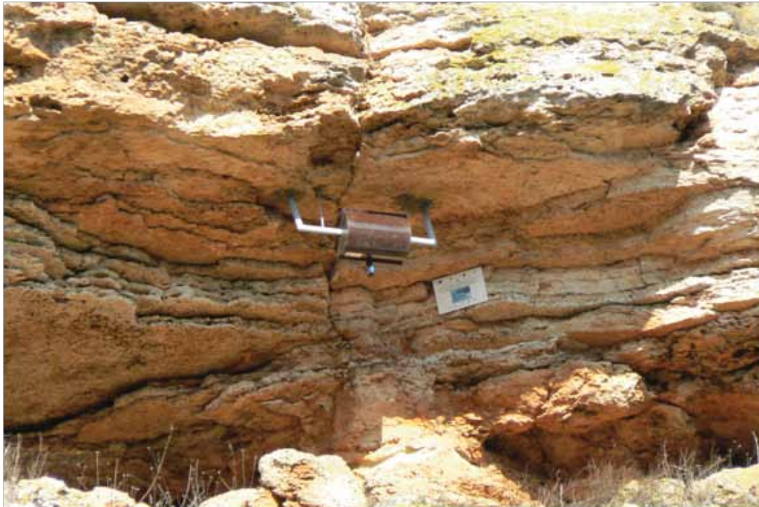
Photo 6 – Extensometer - Cape Kaliakra, Bulgaria
