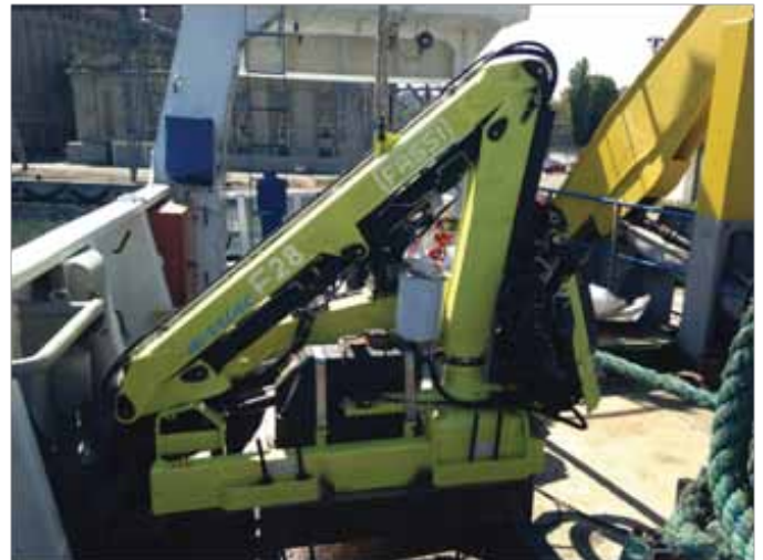
Photo 8 – Crane for guns deployment
