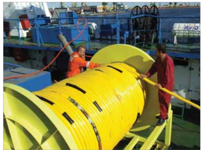
Photo 10 – Spooling the seismic streamer on winch
